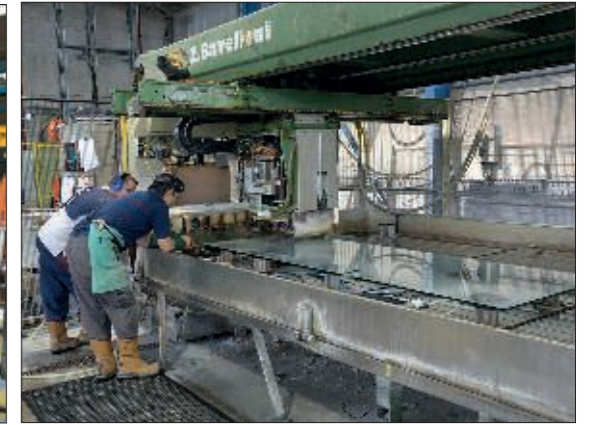
On its CNC processing machines incorporated completely automatically into the A+W network, FGI manufactures glass for interior applications such as separator walls, tabletops, shower doors, glass door systems, etc.
