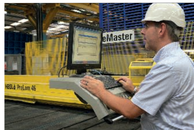
On the HEGLA combi cutting line, it is possible to cut laminated in flexible alternation with float. The remaining sheets are kept in an HEGLA Remaster storage system and incorporated into ongoing production according to the situation by the A+W optimisation.
