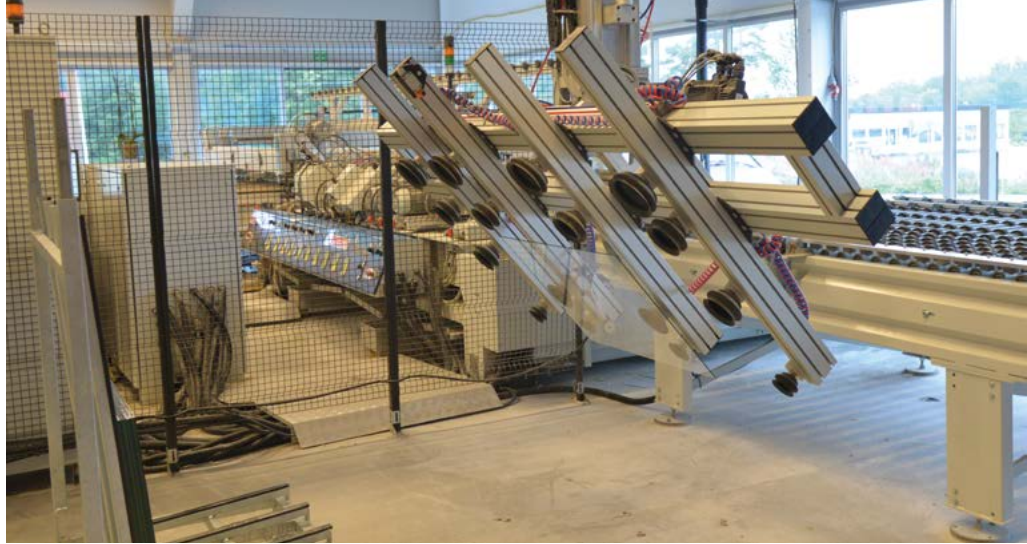
On the path to Industry 4.0: robot loading the double-sided automatic edging machine.
