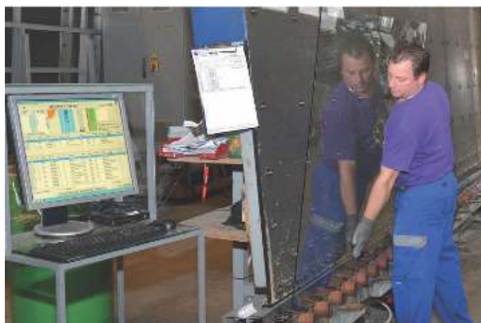
The A+W Production Monitor at the IG line entry shows the sheet structure, position of layers, and reference edge.
