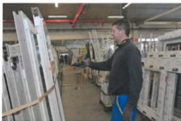
Production information is read out using bar code readers and, as here, status information is reported back to the A+W CANTOR system.
