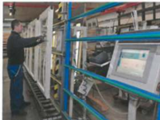
Which pane belongs with which sash? Clear information per monitor on the glazing line.
