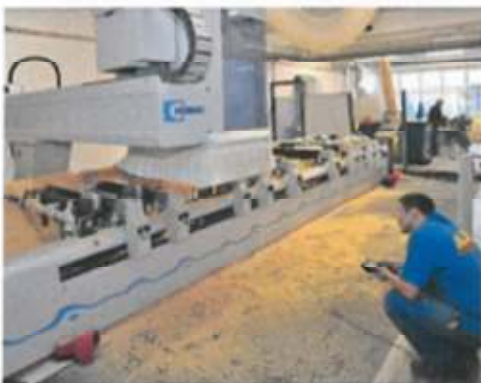
The state-of-the-art Homag CNC wood-machining center for top-quality profiles is controlled by A+W CANTOR software. 90 mm profiles are standard for AJM wood windows.
