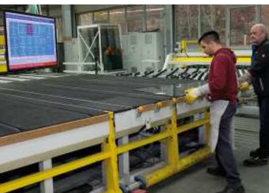
A+W Production Monitor on the cutting table
