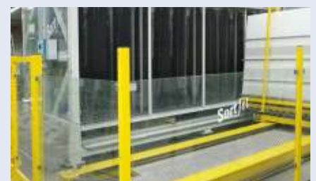
HEGLA SortJet with online connection to the insulated glass line: now even more efficient with A+W DynOpt II
