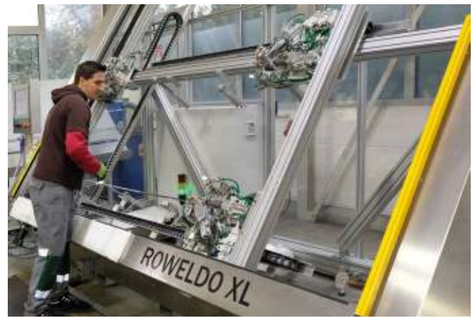
Left: Special insulated glass line for the production of high-quality door inserts with up to 4-layer insulated glass Above: Automatic welding of Swisspacer spacer frames
