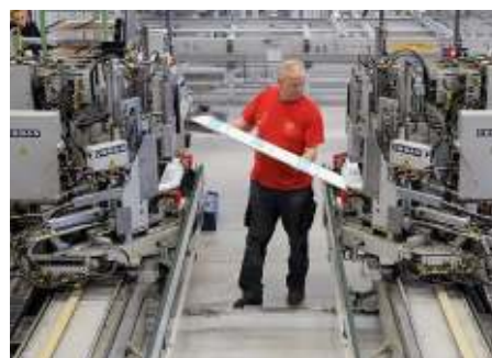
A+W Cantor CIM reliably informs the machine operators on the welding machines which profiles they must insert
