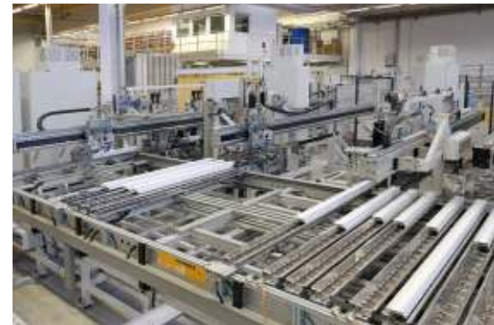
The completely automatic Schirmer processing center handles all processings on the bars and then stacks processed profiles in slot carts
