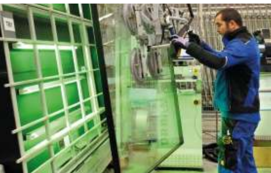
On intake of the insulated glass units into the glass buffer, each sheet is assigned a fixed position. Prior to this, there is careful quality control
