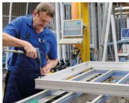
An A+W Cantor CIM-monitor in special construction: at LÖWE, most production workstations are networked
