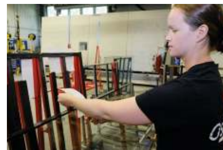
IG unit produced and packed on shipping rack: The barcode label contains all critical lite information
