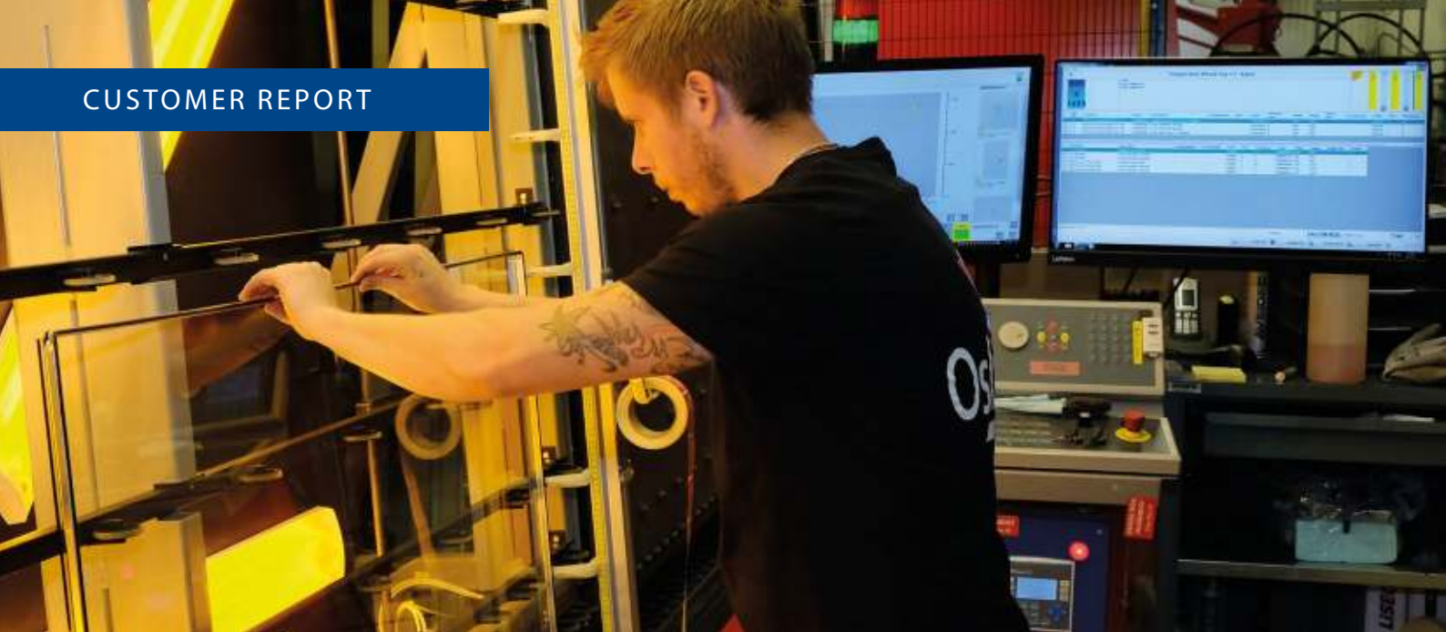
Correct lite? Correct orientation? At the visual inspection station, A+W Production Terminal helps workers assemble insulated glass units flawlessly
