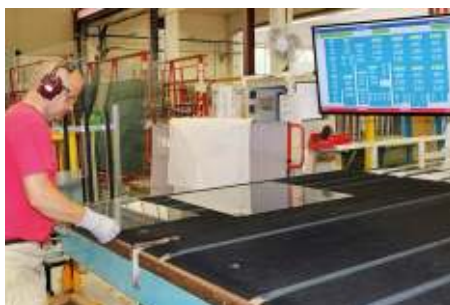
Perfectly optimized: The A+W Production Monitor clearly shows the break pattern and storage location in float cutting
